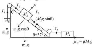
$$T_1 = T_2 + M_2 g \sin(37^\circ) + \mu M_2 g \cos 37^\circ$$
