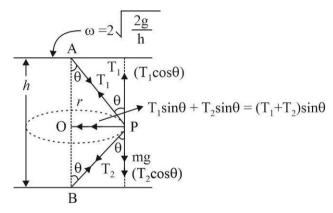
$$\frac{\left(T_1 + T_2\right)}{\left(T_1 - T_2\right)} = \frac{\omega^2 h}{2g} = \left(4 \times \frac{2g}{h}\right) \times \frac{h}{2g} \quad \left(\text{As, } \omega = 2\sqrt{2g/h}\right)$$
